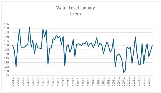
In this graph, you can see the water level measurements for January in the period from 1941 to 2022. The highest water level of January was reached in 1951, with an approximate height of 151 cm. In comparison, the lowest water level of January was observed in 2007, with a height of 98 cm. A significant difference can be seen from these results.<sup>93</sup>
