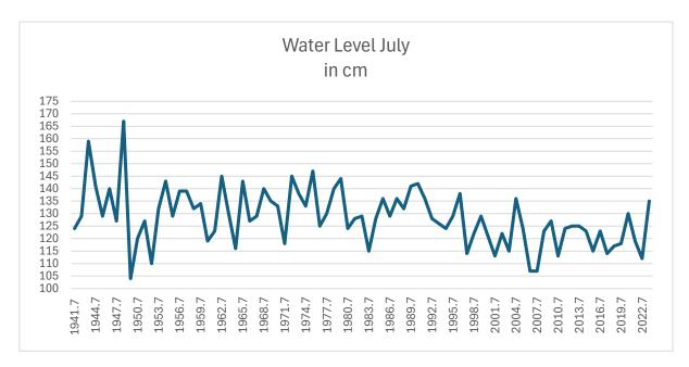
This graph shows the July water level measurements from 1941 to 2022. The highest value was observed in 1948 with a water level of 167 cm. In 1949, the lake had the lowest water level of 104 cm, which is a large difference within one year. This data provided invaluable insights into the complex temporal changes in the water levels of Lake Woerthersee during the period in question.
