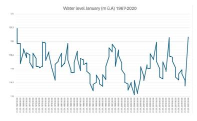
The water level above sea level was approximately 118m-120.5m. The lowest water level was observed in 2004 (118,01 meters above sea level) and the highest in 1967 (120.5 meters above sea level).
